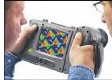
**Camera Performance:** The camera shall have a minimum resolution of 1°C (1.8°F)
