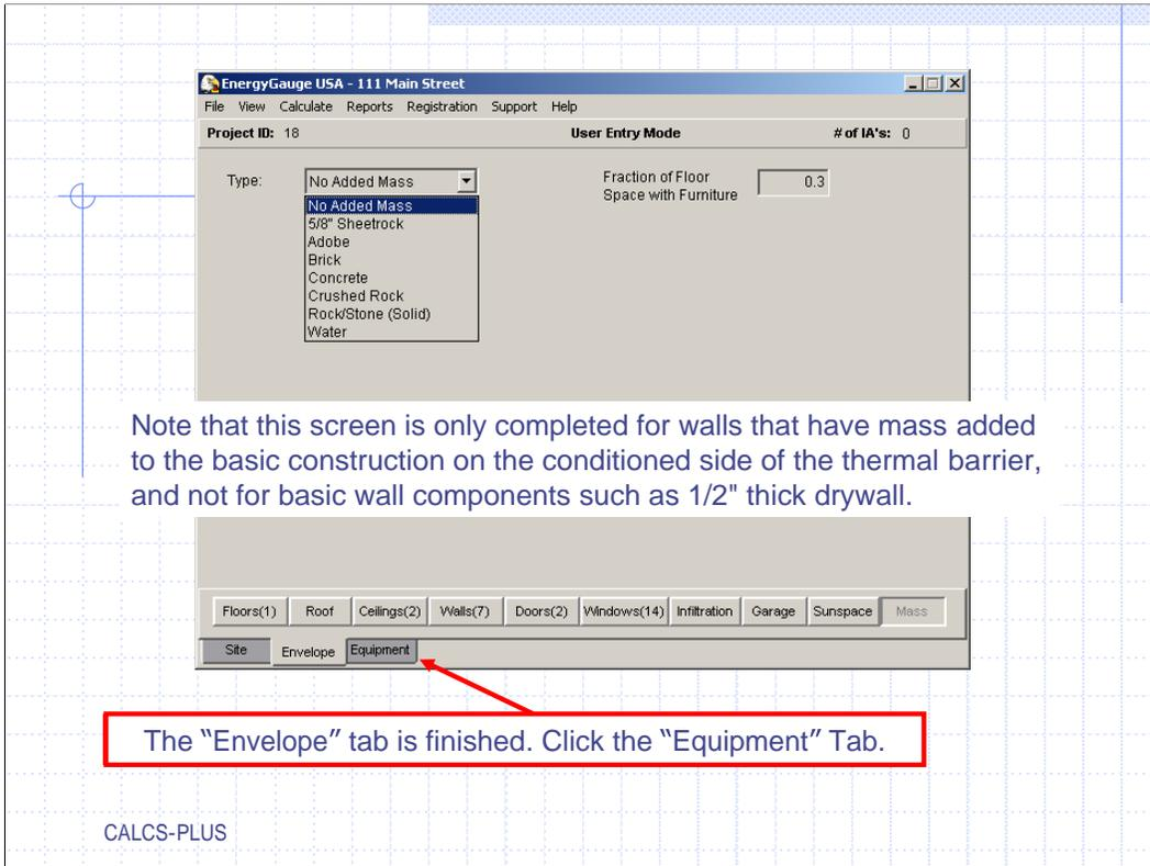
Note that this screen is only completed for walls that have mass added to the basic construction on the conditioned side of the thermal barrier, and not for basic wall components such as 1/2" thick drywall.
