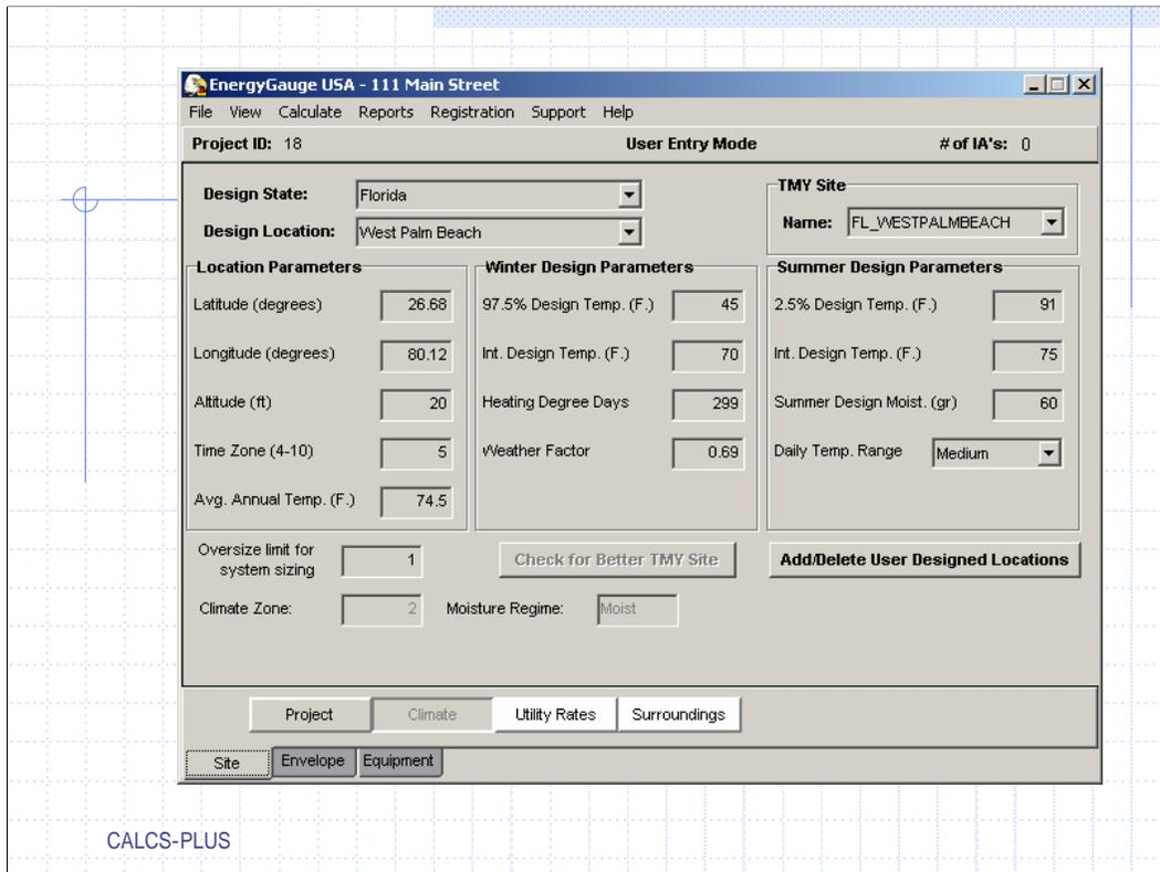
RHVAC does not transfer climate information so this screen must be edited or you may find your project in Anchorage Alaska. Select the climate for this job. The same data base that was in the Load Calculation program is in the rating software. Return to project page and save.
