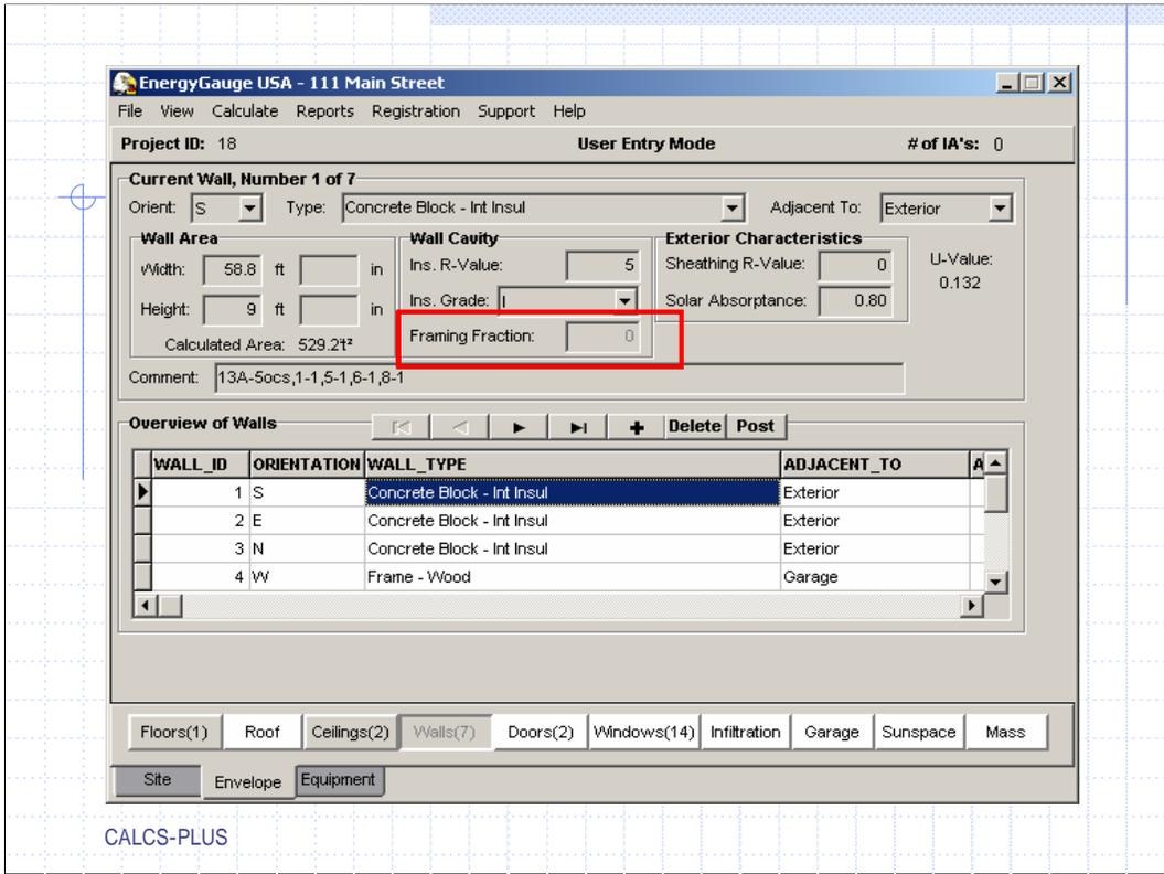
USA looks at “Concrete Block – Int Insul” or “Concrete Block – Ext Insul” walls as having continuous insulation with no framing factor.
