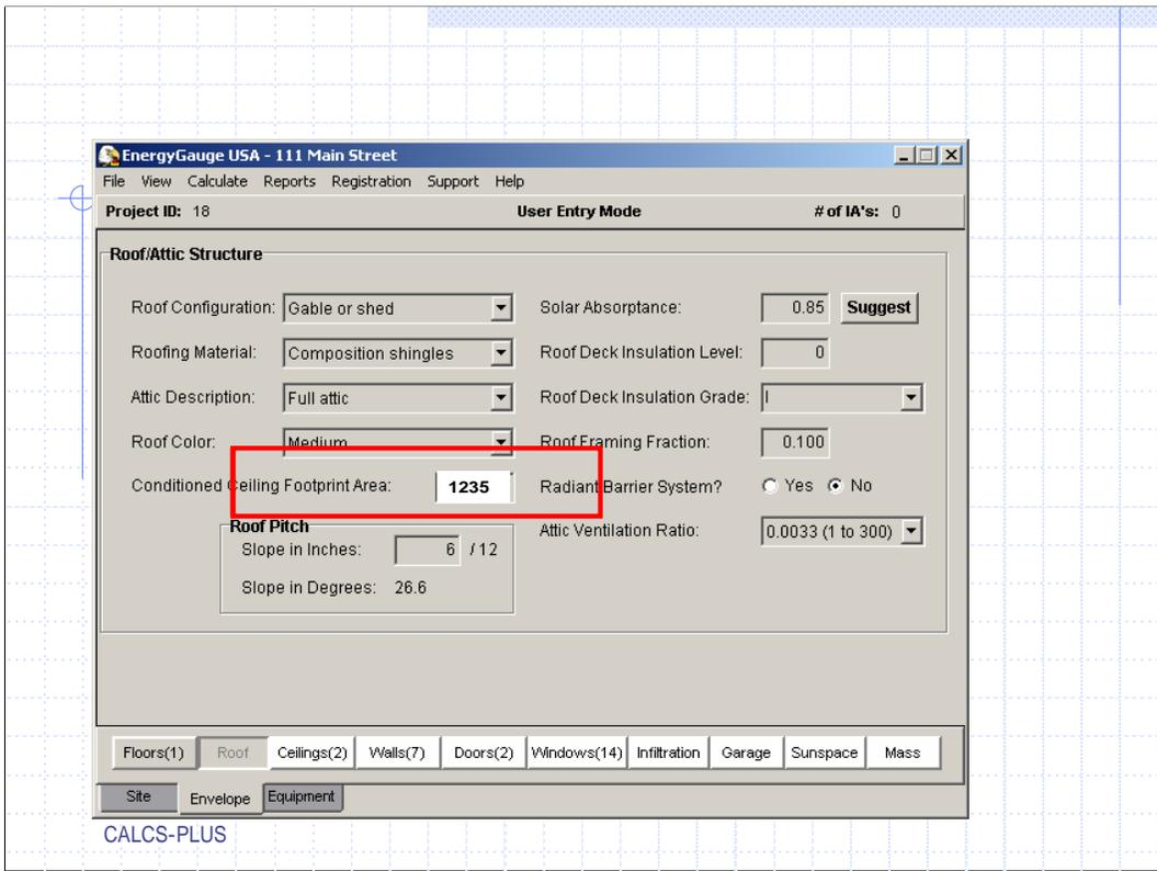
Note: If it is a single story home the floor area under ceiling is the same as the SQ FT of the home. The conditioned ceiling area may be larger, especially if we are dealing with tray or cathedral ceilings. Change the roof configuration, materials, etc to match your building.
