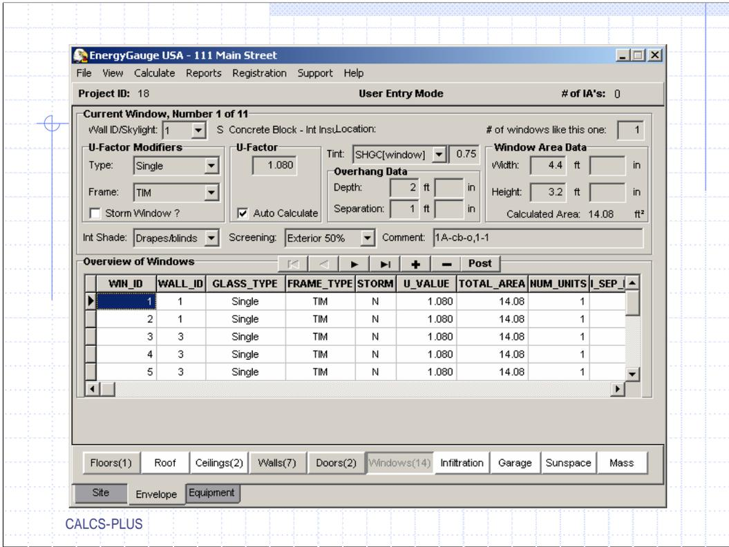
Windows transfer from the load calculation program as they were entered; the window height and width; the overhang depth and separation; interior shading, and screening all come into USA with no editing necessary. As on the wall page, the “Comment” box tells the type of window, room & wall the window is on in RHVAC.
