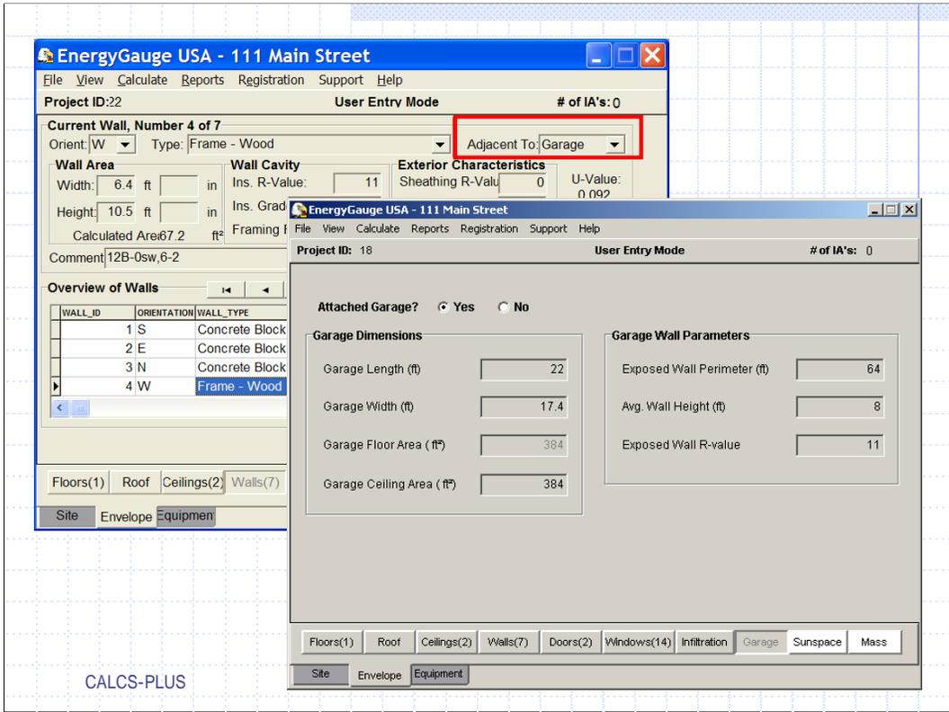
RHVAC automatically builds a default garage in USA, this is needed because back in the wall section we had some walls that were “Adjacent To” a garage. If all the walls are “Adjacent To” Exterior you can click on “No”. But in this example we have an attached garage and since RHVAC exported a default garage we can edit to the proper dimensions.
