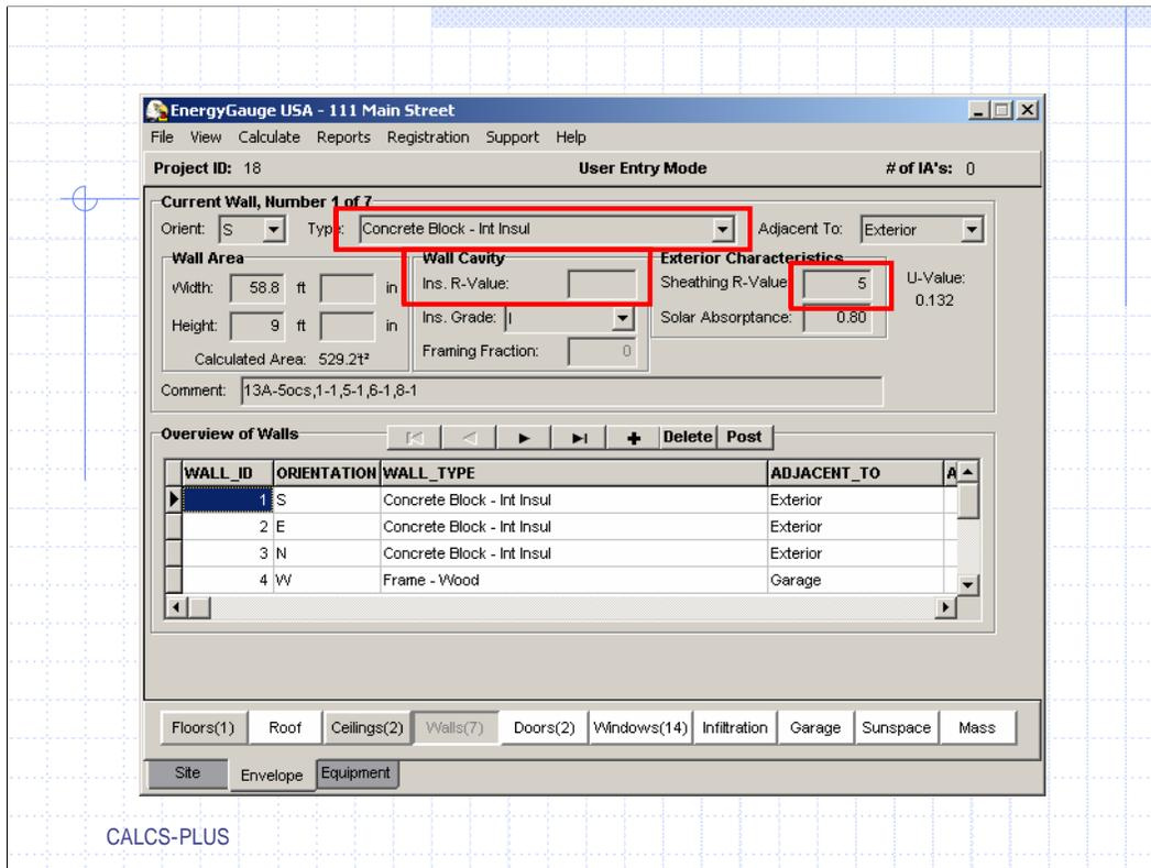
Our wall information comes in correct for direction and SQ FT. This wall transfers over as a “Concrete Block –Internal Insulation”, note that under “Wall Cavity” the “Ins. R-Value” is 0 and under “Exterior Characteristics” the “Sheathing R-Value” is 5, this will need to be reversed to match the construction type of the project we are working on.
