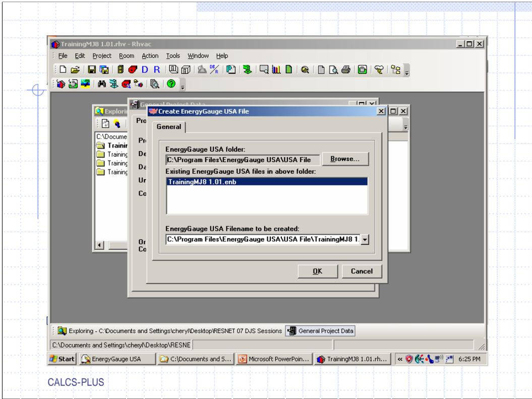
Energy Gauge USA uses a .enb file. We keep these files in a separate folder on our computer and re name them when we open them in our rating software, after the rating is complete we file them in a folder under the builder's name.
