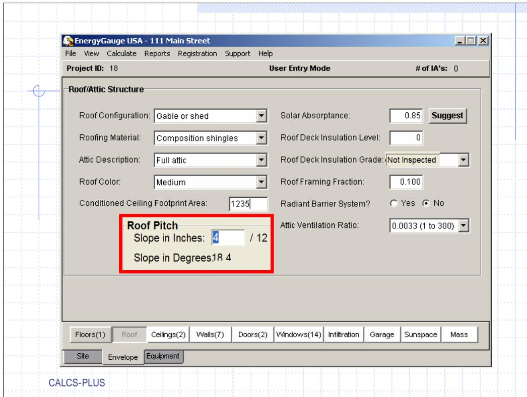
The “Roof Pitch” defaults to 6/12, change the roof pitch to match the home you are working on.
