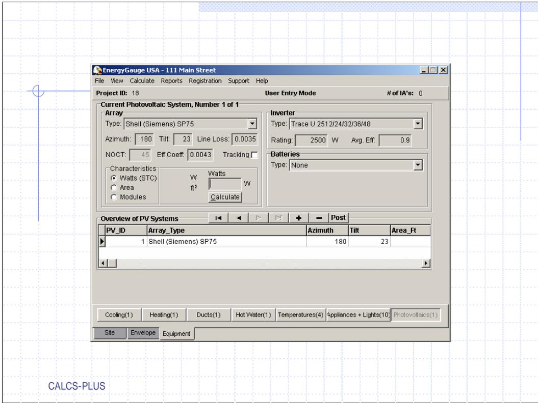
Photovoltaic Systems can be added here. Verify the information for the system at your building
