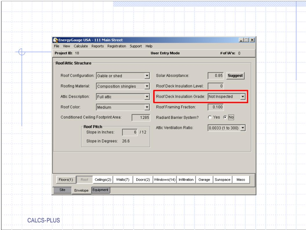
If the roof has insulation on the deck then select the insulation grade, click the down arrow for “Roof Deck Insulation Grade” if this is a projected rating from plans choose “ Not Inspected”. Now is a good time to save your project.
