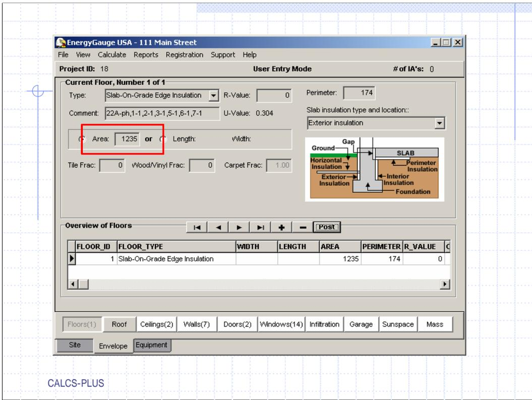
The information we entered into the load calculation program has transferred into the floor tab, this is as we entered it. Remember on the “Site” tab we changed the square foot of living space as recorded on the plans by the builder. On this screen the total floor area should be the same as the “Conditioned Ceiling Footprint Area ” under the “Roof” tab.
