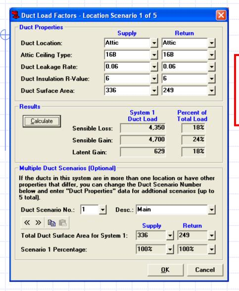
The Sensible Loss, Sensible Gain, and the Latent Gain are calculated for the duct system.
