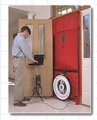
Energy Raters use controlled airflow to estimate the amount of uncontrolled airflow.
